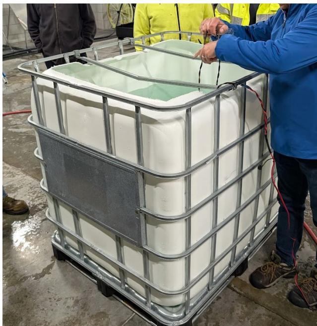
Figure 15. Intermediate Bulk Container with Top Removed
