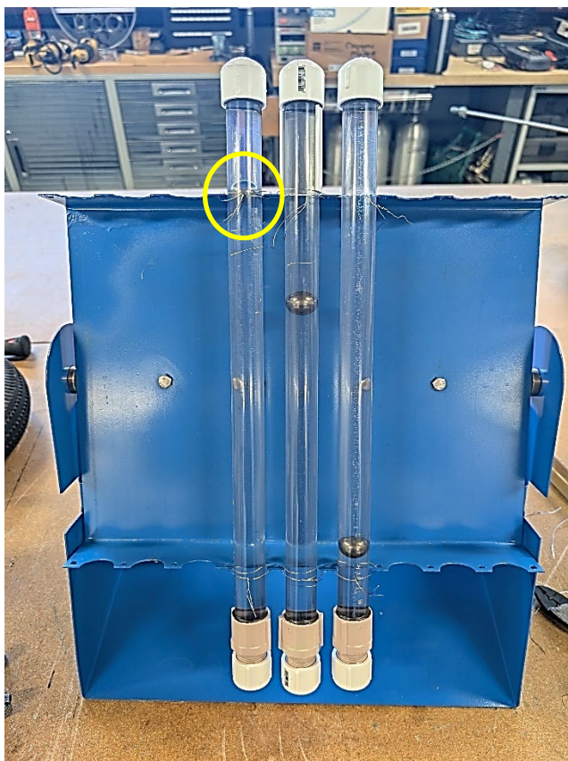
Figure 23. Temperature Effect Evaluation for Surrogates Using Falling Ball Viscometers (Note the ball in the left viscometer is circled in yellow to show its position.)
