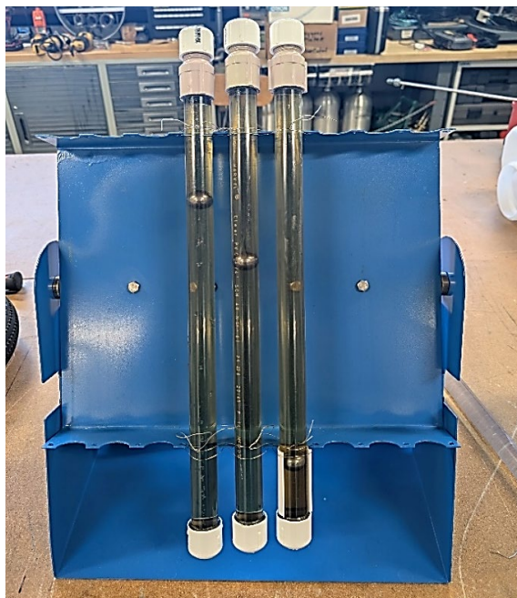
Figure 22. Temperature Effect Evaluation for F3 Using Falling Ball Viscometers
