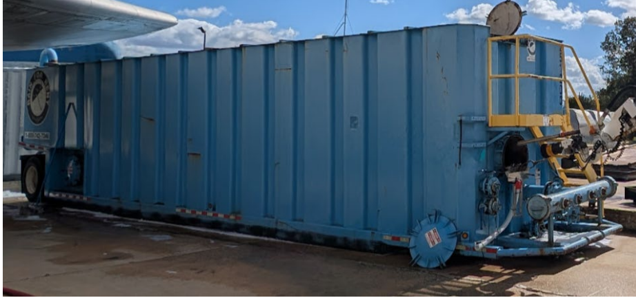
Figure 7. The 21,000-Gallon, Flat-Top, Corrugated Wall Tank
