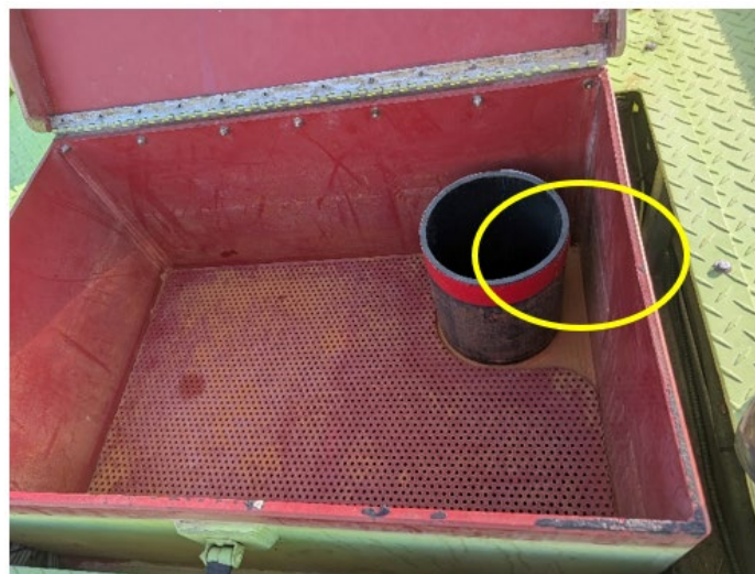
Figure 20. Water Tank Pre-Marked Stop Line
