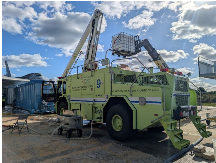
Figure 19. Positioning of Equipment for Output-Based Testing
