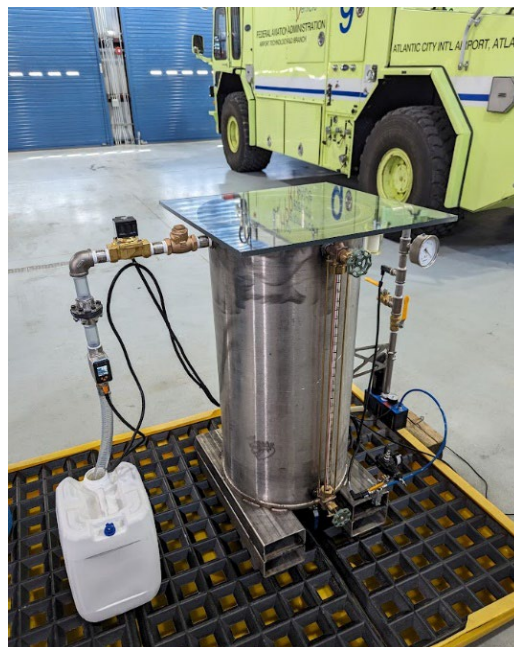
Figure 1. Custom-Built, Vacuum-Based Testing Fixture
