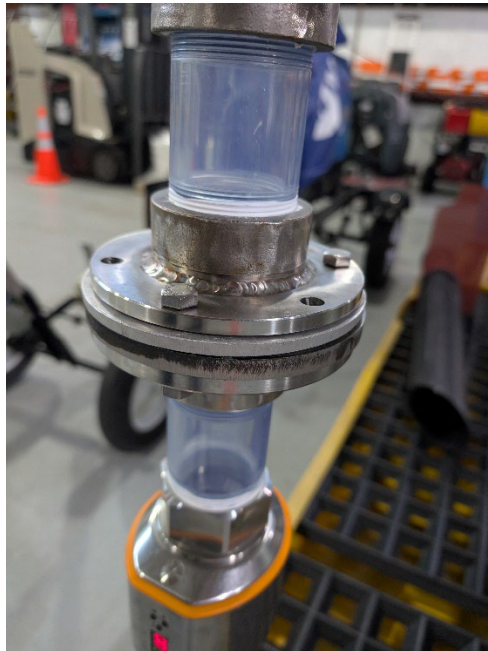
Figure 17. Orifice Plate Holder and Clear Intake Tubing
