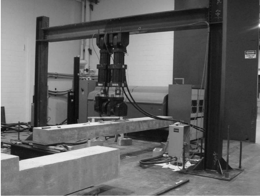
Figure 1-43 Center load reaction frame (Axial load frame not shown)
