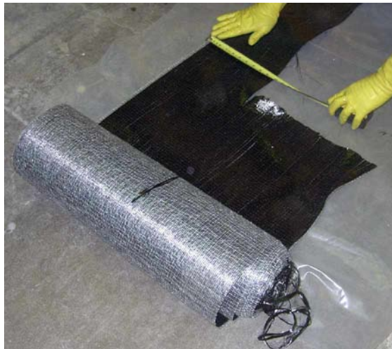
Figure 2-13 Tyfo SCH-41 roll sheet
