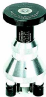
Figure 2-19 The pull-off test apparatus
