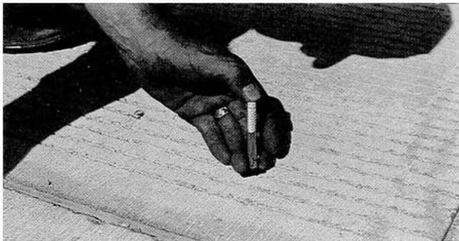
Photo 23: Texture depth measurement using a tire tread depth gauge
