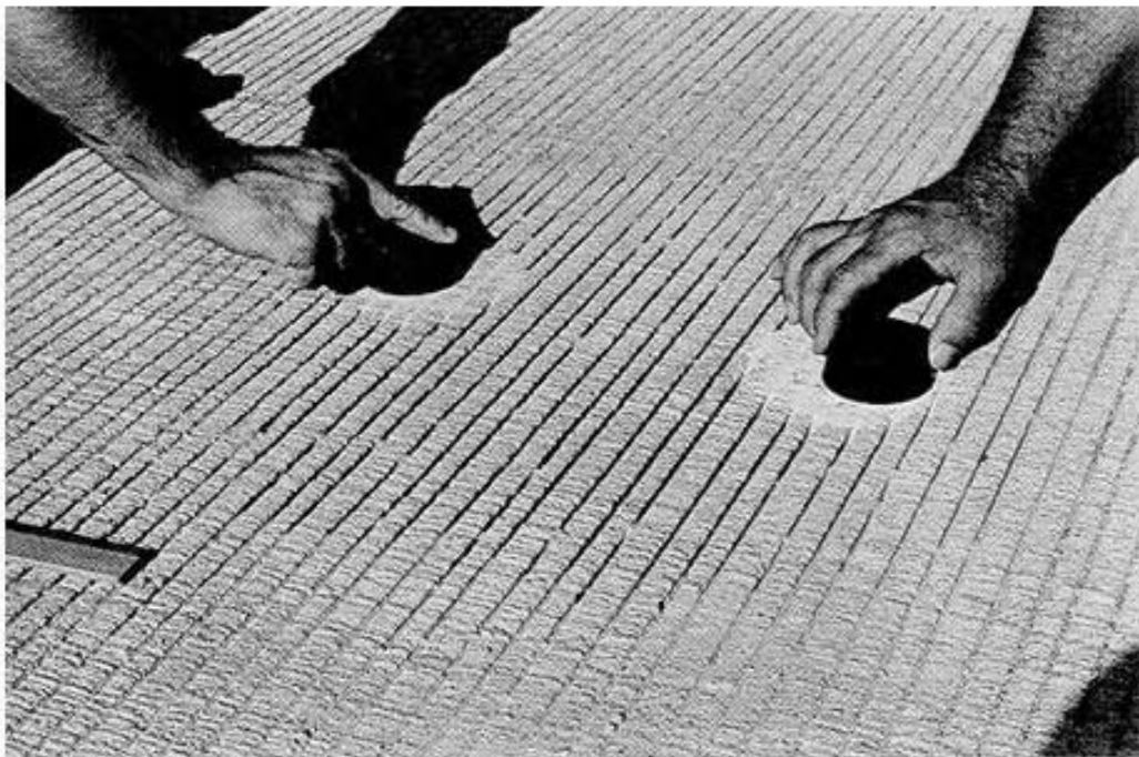
Photo 22: Sand patch test for measuring texture depth
