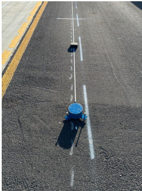
Figure 38. Photo. BP guide tape at a test section lead-in.
