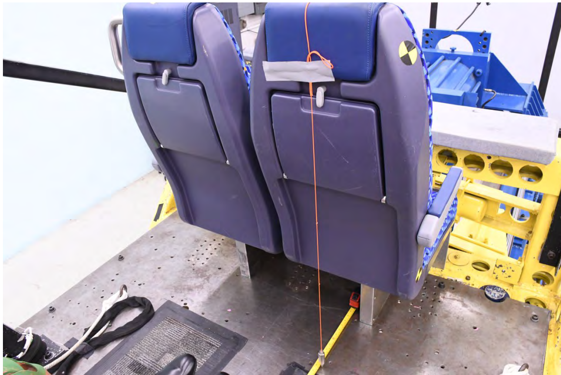
Figure A52. VP2409 Pre-test View of Plumb bob Set Up
