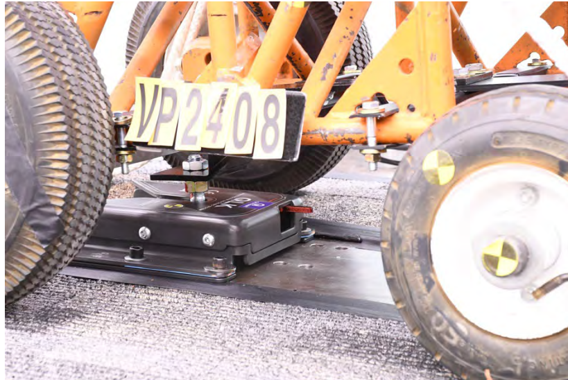
Figure 4. Q'Straint QLK™ docking hardware, as used on the test wheelchair
