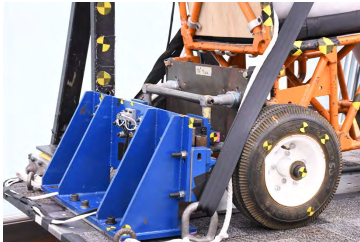
Figure 3. Example of the UDIG on the Wheelchair Test Fixture
