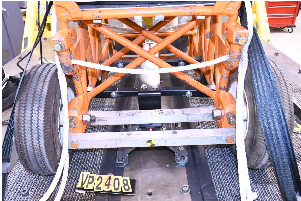
Figure A31. VP2408 Pre-test Rear View of QLK™ Dock and Stabilizer Bracket
