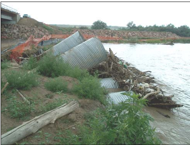
Figure 1.5. View of failed Pinon Bridge detour culverts on Fountain Creek. Spring 2004 (CDOT Region 2).
