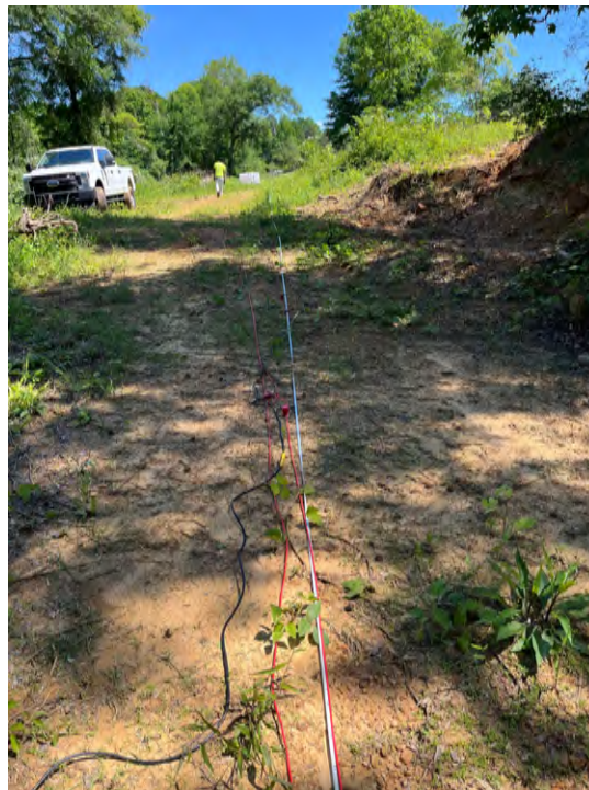
Figure 43: Seismic survey line at Duck River site
