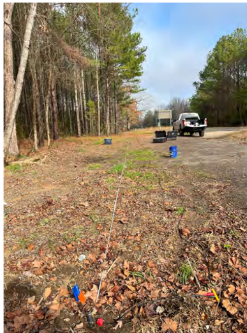
Figure 29: Cedar Bluff MASW survey line
