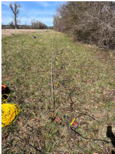
Figure 41: Greensboro seismic survey line
