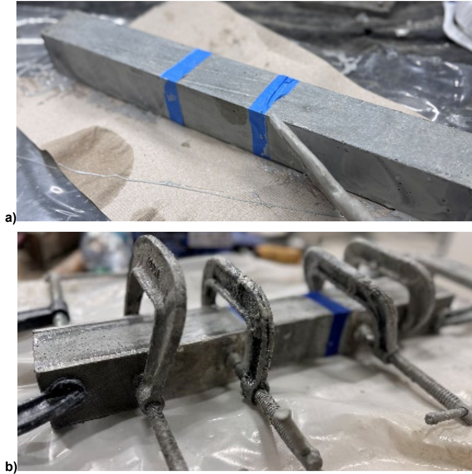
Figure 4-2: Image Showing a) Thin Layer of Epoxy Applied to the Cleaned Surface and b) the Aluminum Plates Held in Place by Three C-Clamps at Each End (blue painters tape added for ease of cleanup)
