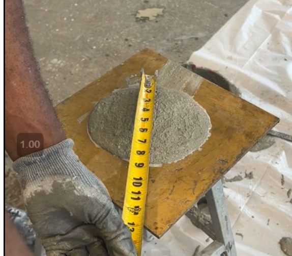
Figure 6-9: Flow Test Being Performed
