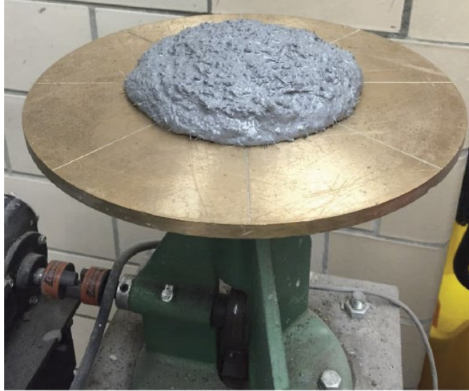
Figure 2-5: Example of UHPC Flow Test (ACI 239R 2018)
