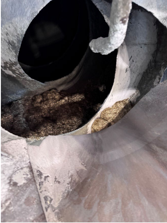
Figure 6-7: Steel Fibers in the Truck
