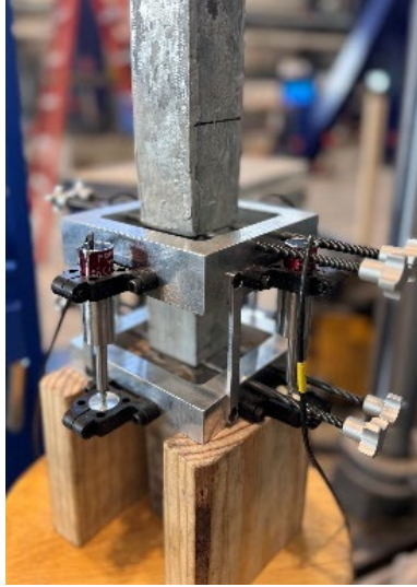
Figure 4-3: Image Showing the Alignment of the Deformation Measuring Device
