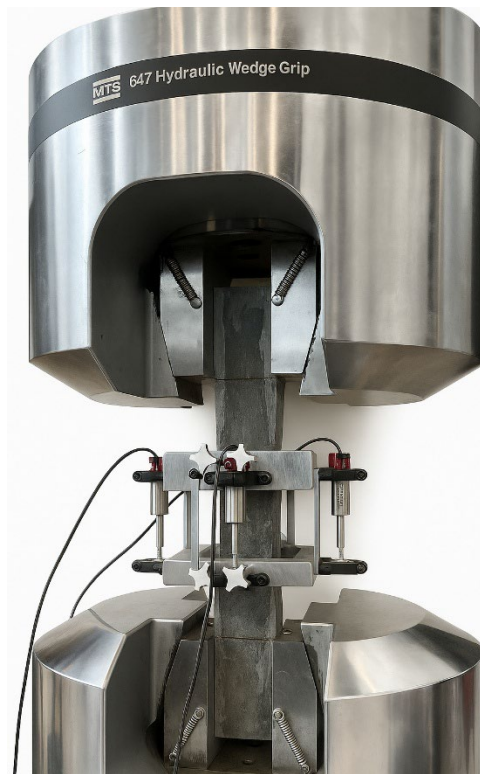
Figure 3-8: Typical Uniaxial Tensile Test Setup for Auburn University UHPC Testing
