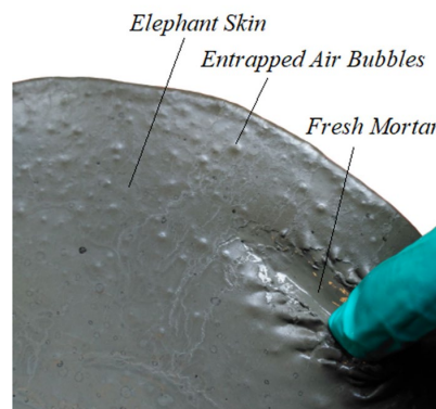
Figure 2-7: Elephant Skin Formation Just After Slump-flow (Yalçinkaya and Çopuroğlu 2021)
