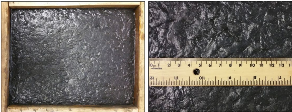
Figure 2-6: Surface Appearance of a Base UHPC Mixture, Depicting Elephant Skin Formation on the Exposed Surface (Chen et al. 2017)
