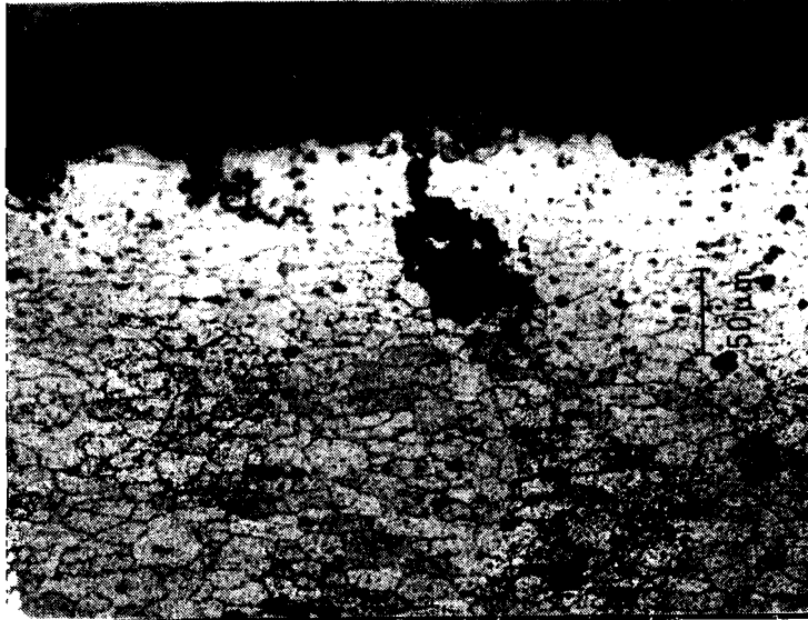
Figure 16. Optical micrograph cross section view of a shot peened specimen 200 magnification.
