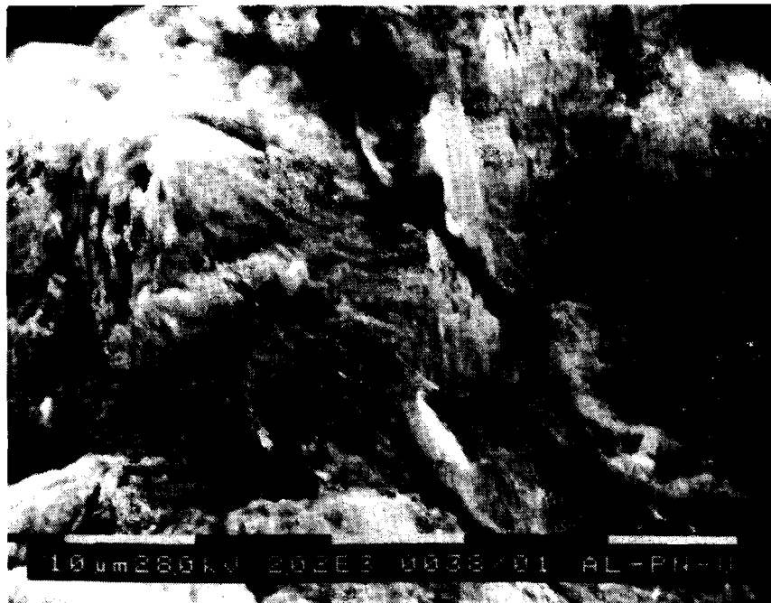
Figure 3 SEM micrographs of surface morphology introduced by the paint removal process impacted with PMB particles traveling at a velocity of 78 m/s, at angles of impingement of (a) 15 degrees and (b) 90 degrees.
