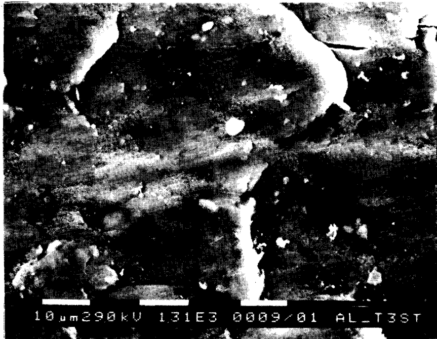
Figure 10. Morphology of the scratch surface after 35,000 cycles, 1300 magnification
