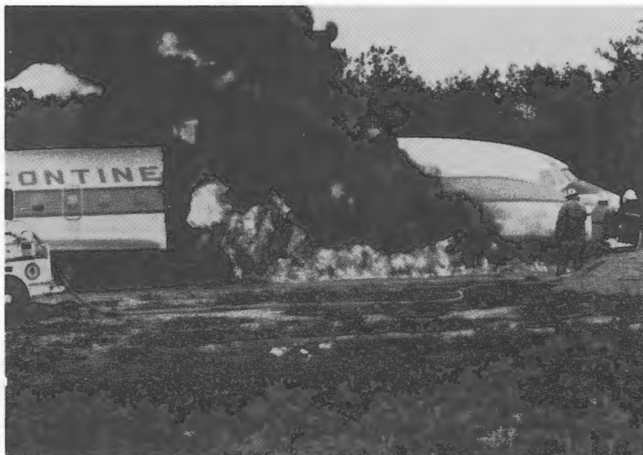
FIGURE 5. TEST 2 DC-8 FLAME EXPOSURE
