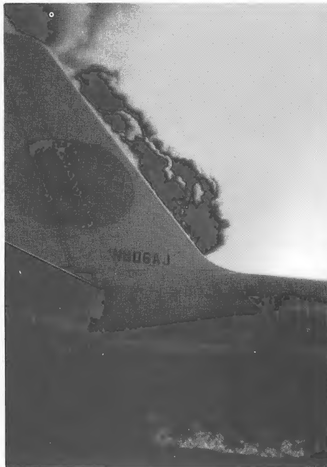
FIGURE 8. TEST 4 CV-800 STARBOARD SIDE FLAME EXPOSURE
