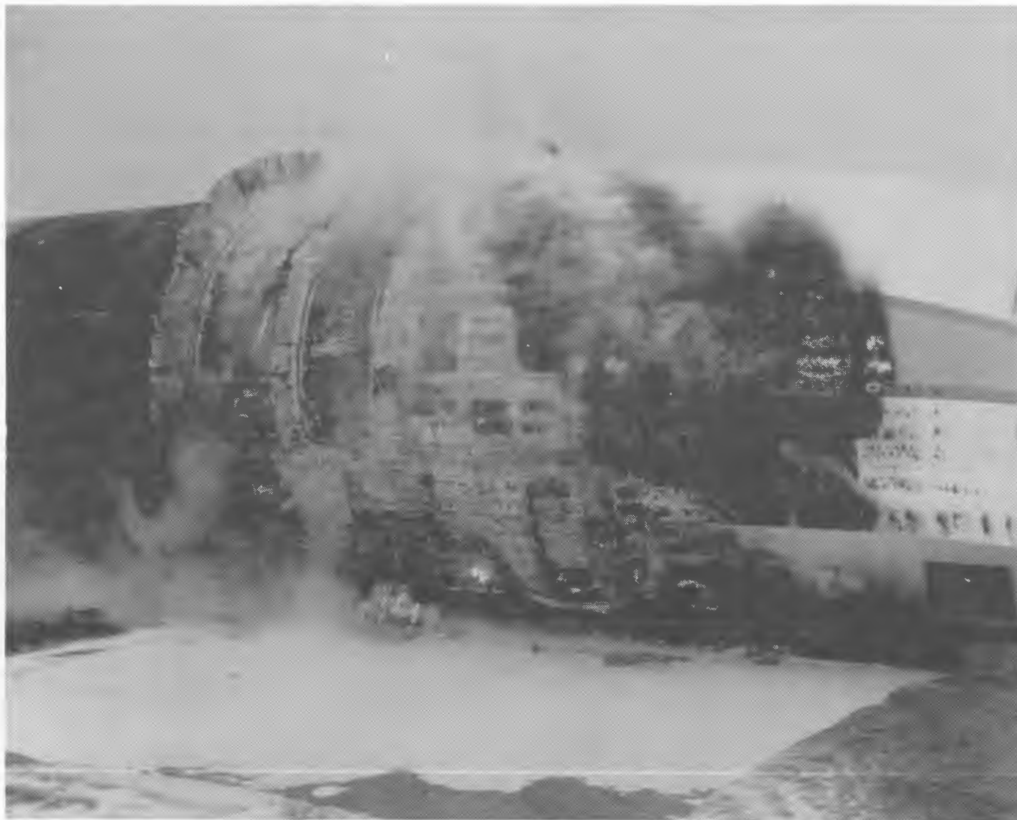
FIGURE B-7. TEST 2 EXTERNAL FIRE DAMAGE, DC-8 FORWARD SECTION
