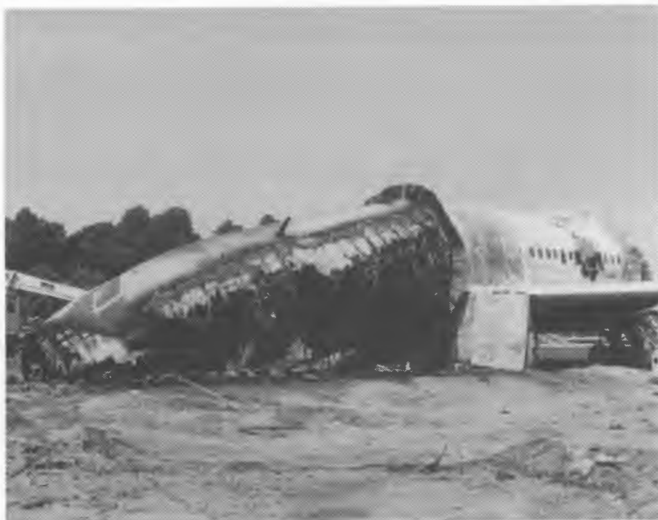
FIGURE 12. TEST 5 CV-880 PORT SIDE FIRE DAMAGE
