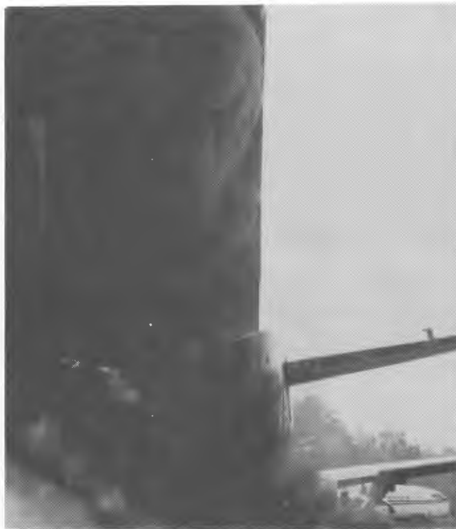
FIGURE 7. TEST 4 CV-880 PORT SIDE FLAME EXPOSURE
