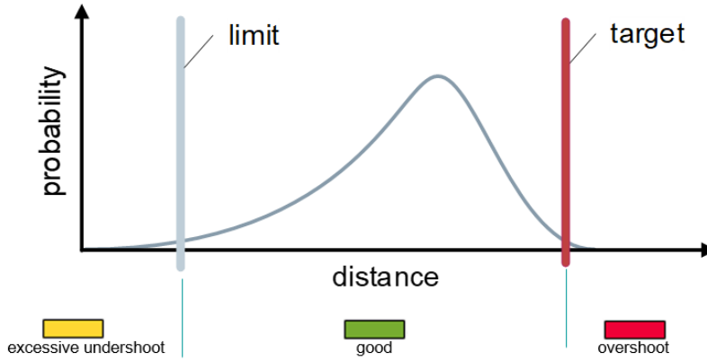
Figure 7. Illustration of summary classification of stopping distance.
