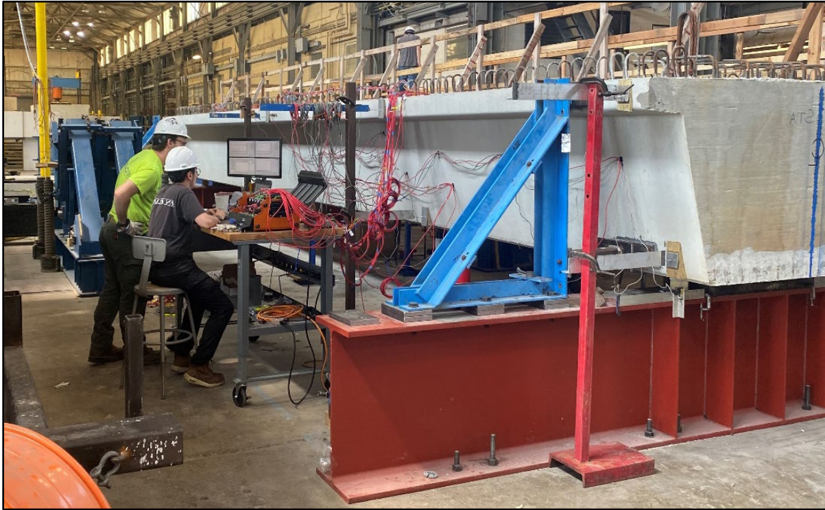
Figure 3.5. Lateral load test of Tx-U40 specimen
