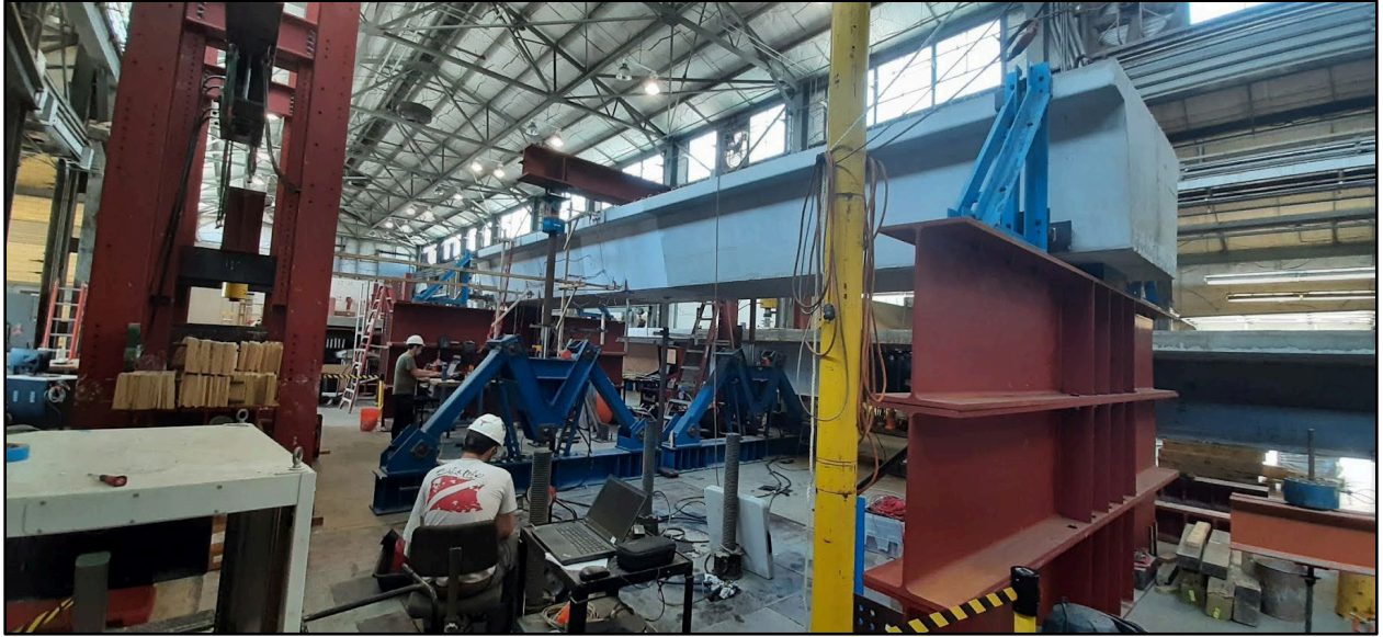
Figure 3.16. Vertical load test of Tx-U40 specimen
