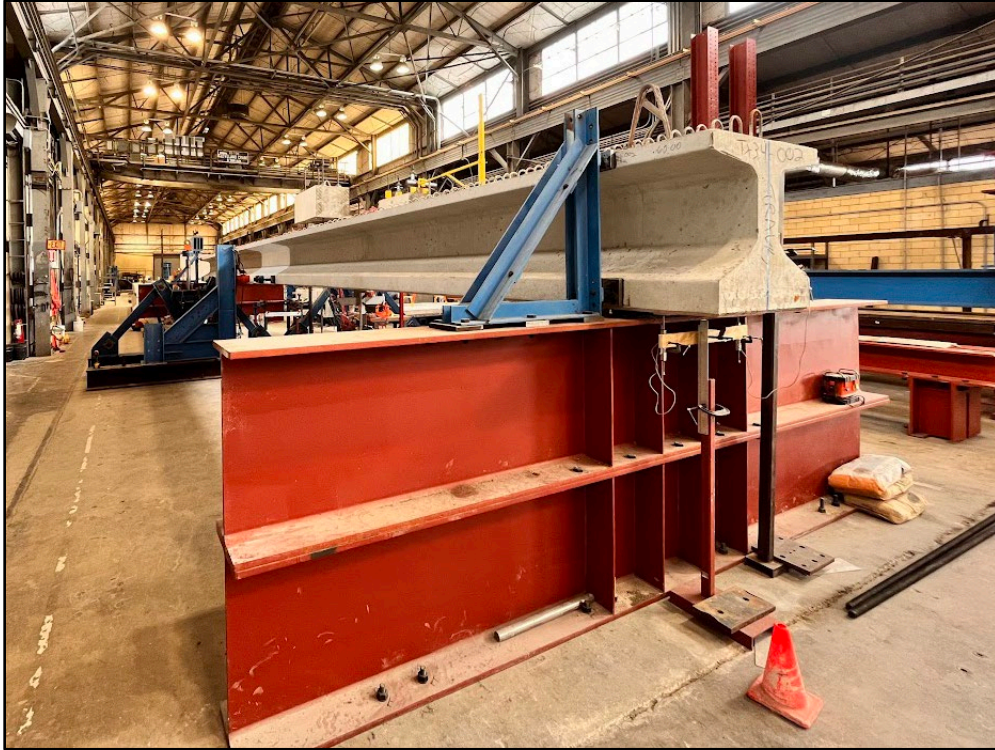
Figure 3.43. Tx34 setup in the lab (Tx28 similar)
