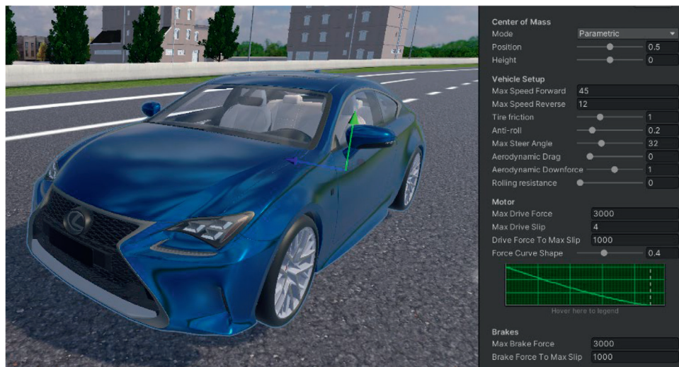
Figure 3.8 Tuning Page for the Vehicle Physics of the Lexus RC.
