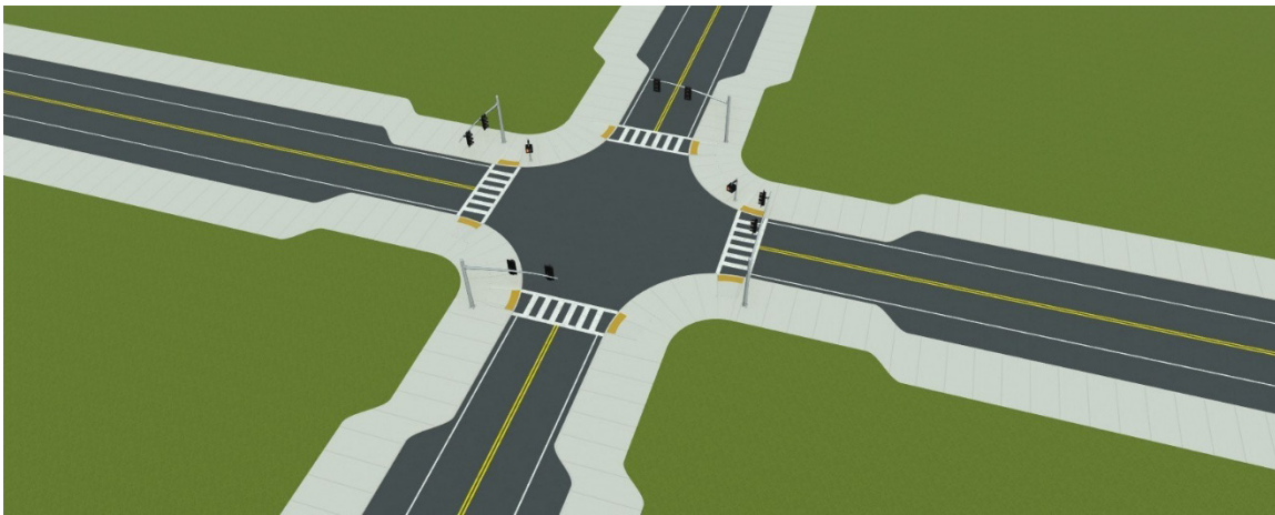
Figure 4.15. Sample Curb Extension Scenario (Aerial View)
