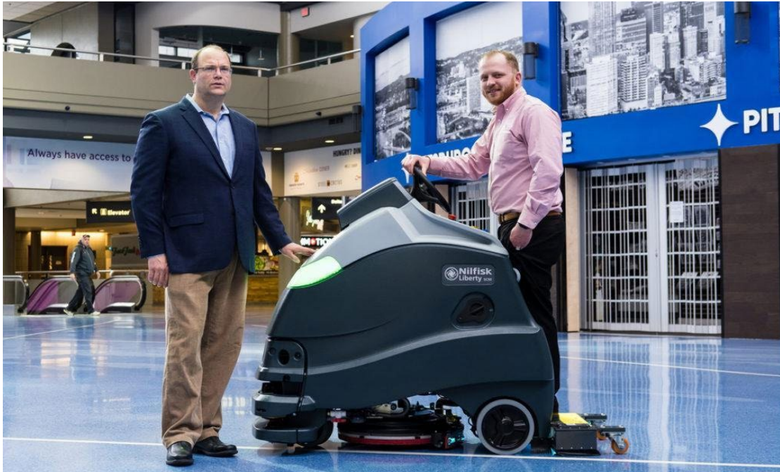
Figure 21. Ultraviolet Scrubber at PIT (Neistein, 2020)
