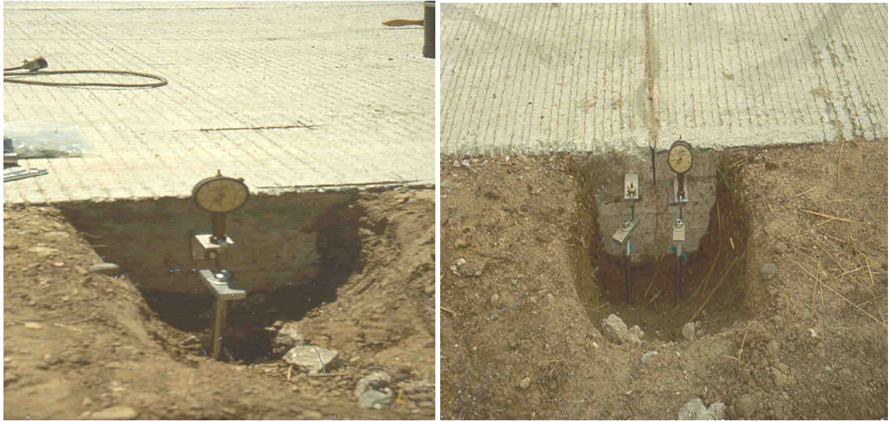
Figures 17 and 18: Acquisition of Curl Data at Mid-Slab and Corners Using Dial Gauges
