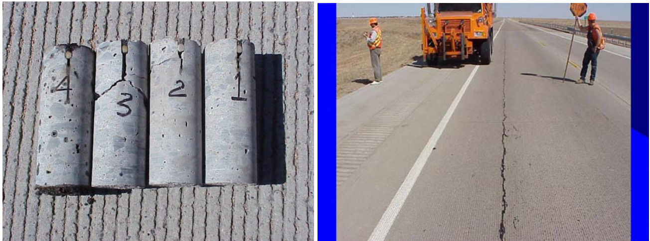
Figure 24: Cores Showing Non-Working Joints
