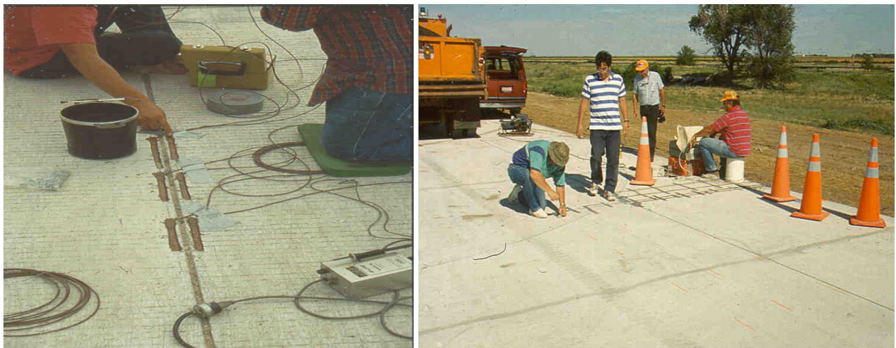
Figures 19 and 20: Surface Mounted Strain Gauges
