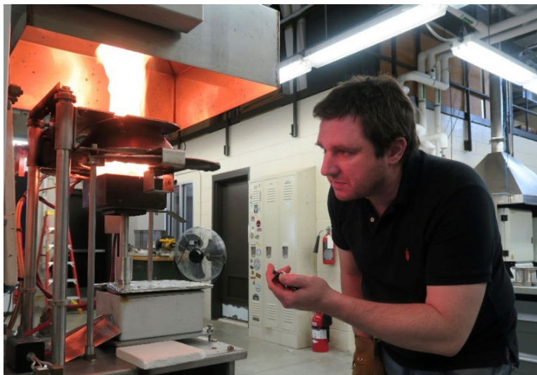
Figure 1. Conducting a test in the cone calorimeter
