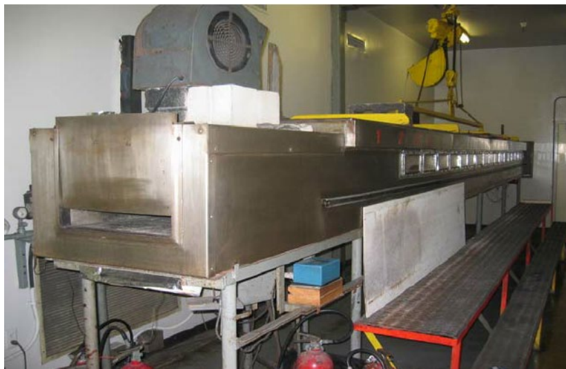
Figure 3. Steiner Tunnel test apparatus (ASTM E84)
