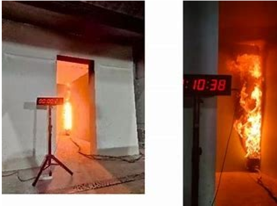
Figure 2. Room corner fire test (ISO 9705) at 0 and 10:38 minutes
