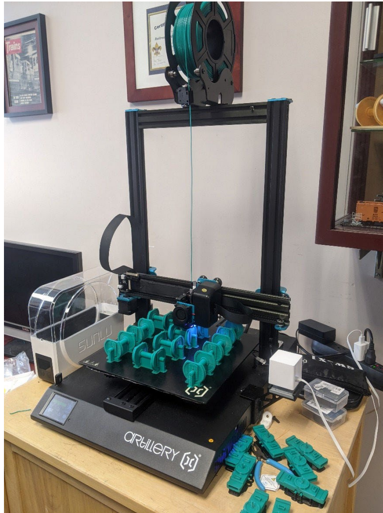
Figure 8. 3D Printing Truck/Bogie Model Components
