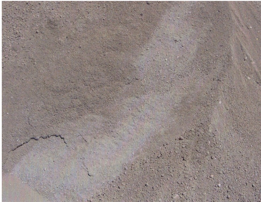
Figure 3. Steel Slag Aggregate Stockpile
