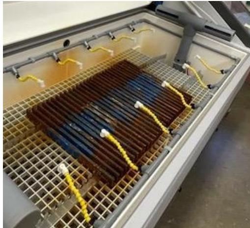
Figure 6. Chloride Exposure Specimens Positioned in the Corrosion Chamber for Conditioning
