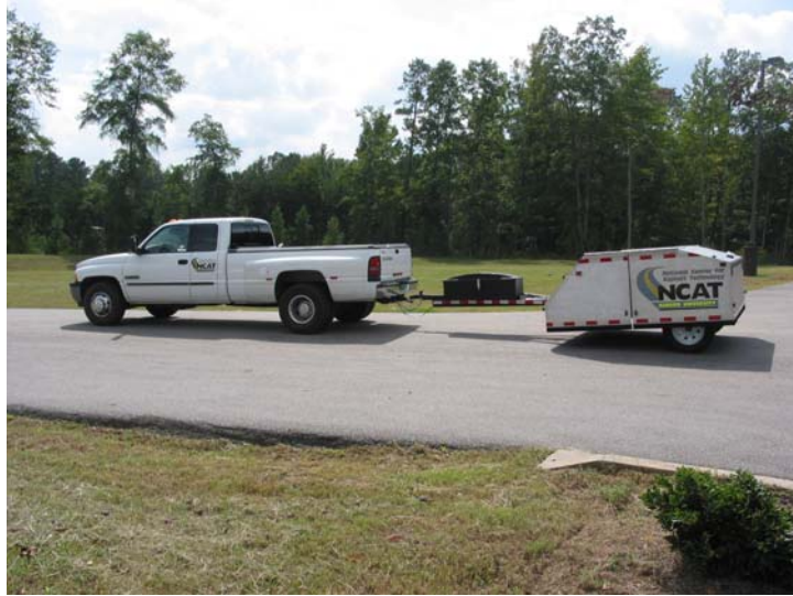
Figure 1. NCAT Close Proximity Trailer
