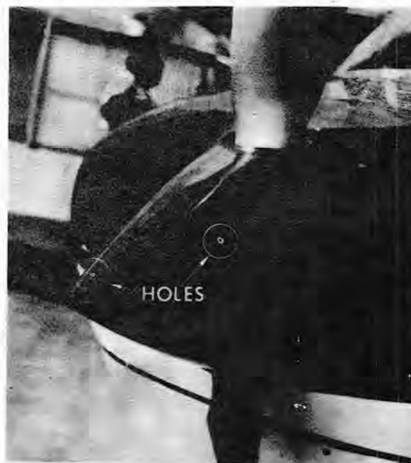
Fig. 4.19 Lightning strike damage to a spinner.
