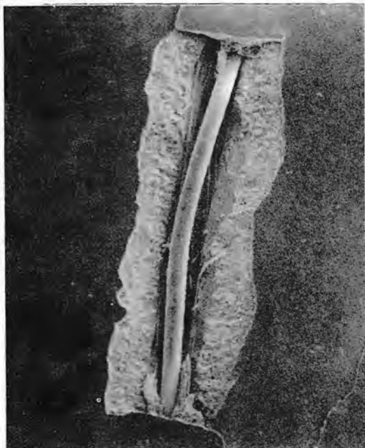
Fig. 6.45 Typical attachment spot on interwoven wire. - 35X magnification
