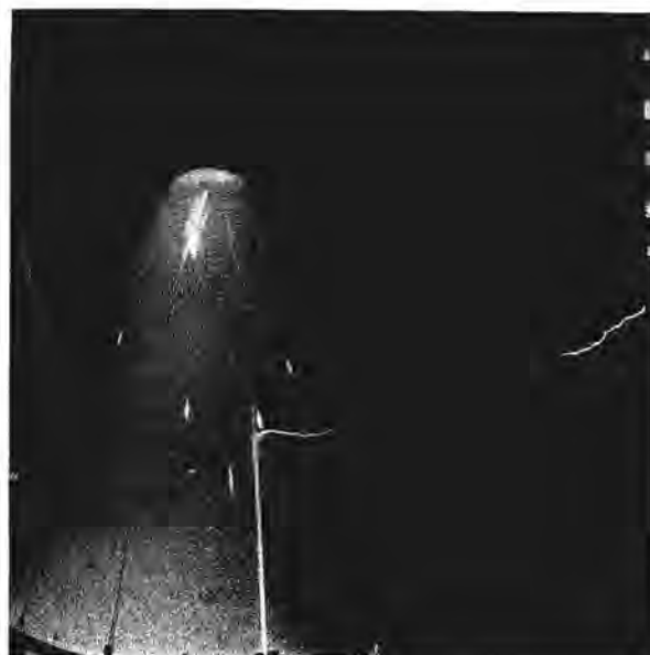
Fig. 6.26 Simulated lightning attachment point tests of a nose radome.
