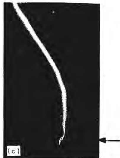
Fig. 2.12 Junction of downward and upward streamers [2.18].
