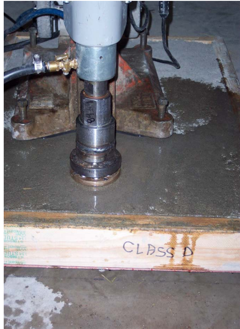
Close-up of custom designed abrasion attachment
