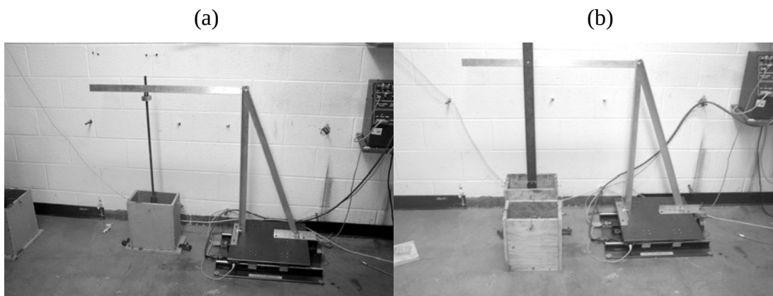
Figure 7: Shake table connected to steel channel in fresh SCC
