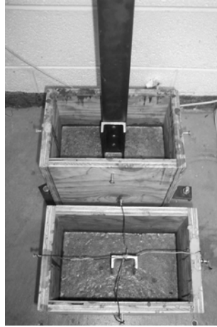
Figure 6: Steel channels in fresh SCC
