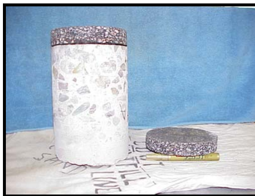
Figure 2: Core sample 4A SMA over PCCP
