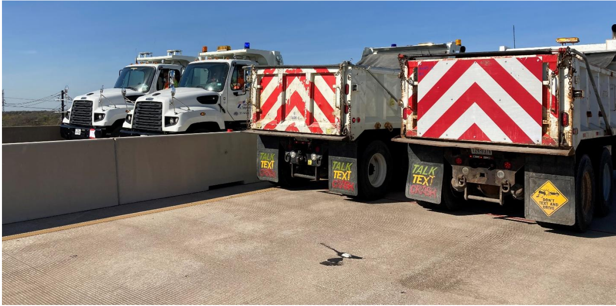
Figure 3-29. Load Case 4 on the Chisholm Trail Bridge
