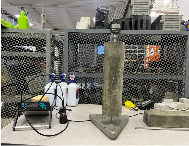
Figure 4.19. Length change measurement using comparator
