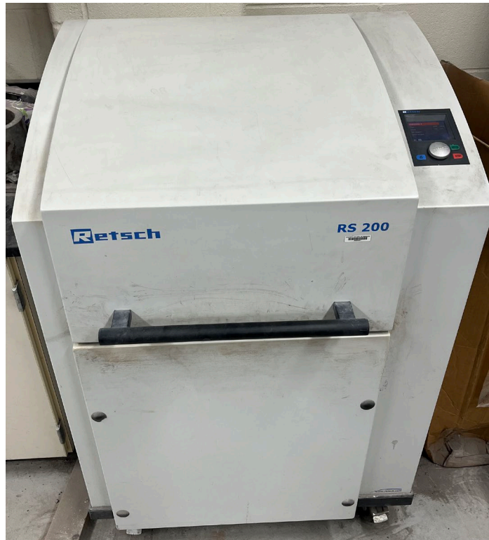
Figure 6.9. Disk mill used for grinding in chloride content determination
