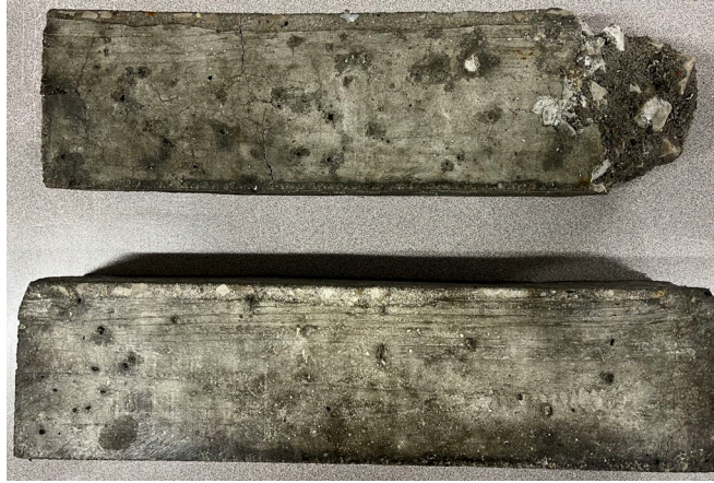
Figure 4.22. Neat silane and silane-nanoclay coated concrete with 5% loading ratio after 200 freeze-thaw cycles
