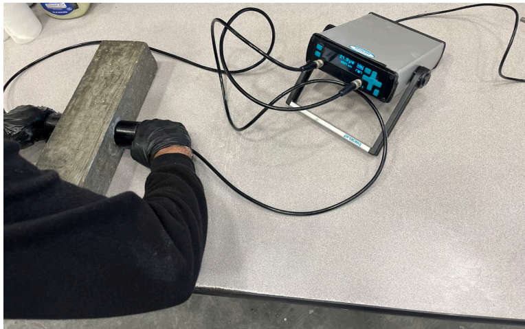
Figure 4.20. Ultra-sound pulse velocity for the determination of the relative dynamic modulus of elasticity
