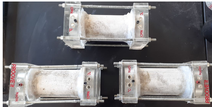
Figure 3.7. Bulk conductivity test measurements
