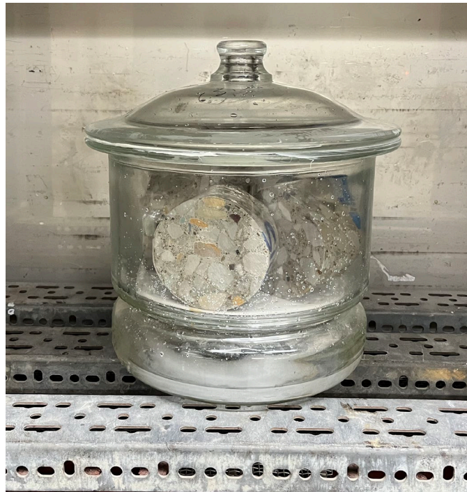
Figure 3.11. Conditioning of the sample using potassium bromide at 120 °F as per ASTM C1585
