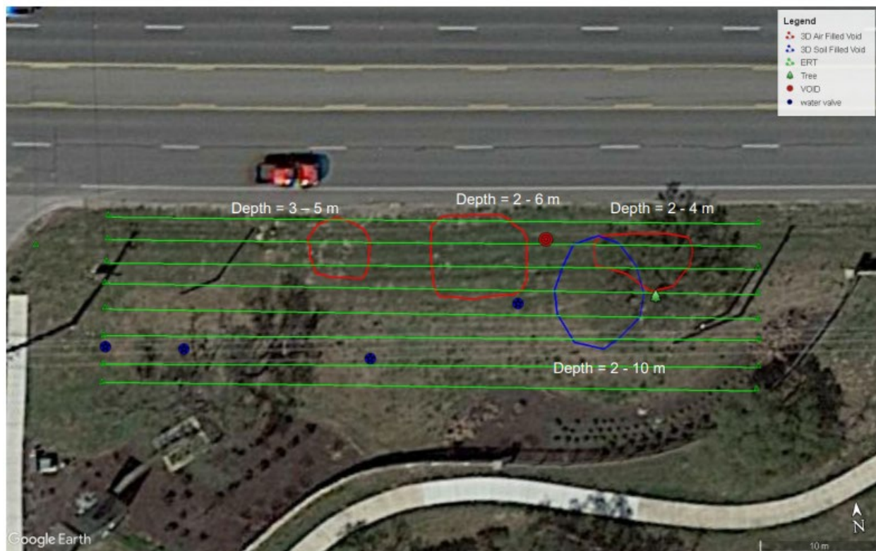
Figure 3.6: Surface map of suspected void locations based on pseudo-3D ERT
