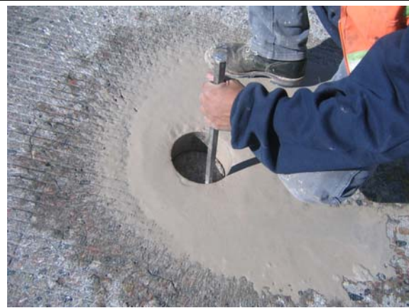
Figure 13 - Coring Concrete Samples on Bridge G-22-BJ. The Core Was Broken in the Traffic Lane
