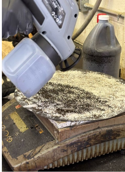
Figure 20. Photo. Use of a spray gun for uniform application of emulsion and a weighing scale to ensure accurate measurement of applied emulsion mass.
