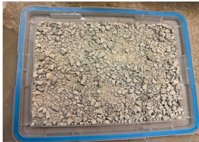
Figure 14. Photo. Board test for calculating aggregate-application rate for modified Kearby method.
