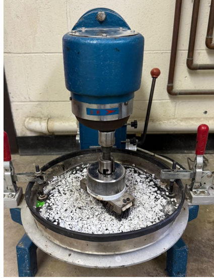
Figure 27. Photo. Sweep-test equipment.
