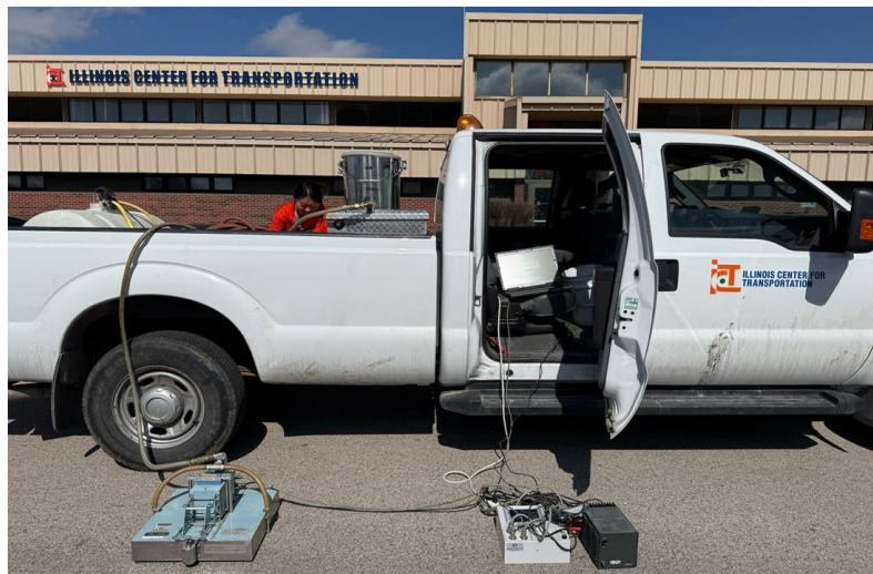
Figure 51. Photo. DFT measurement of asphalt surface at the ICT parking lot.
