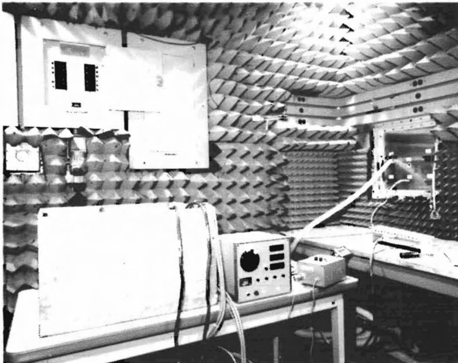
Figure 3-2 Small Shield Room. From Left to Right are Power Supply (in large wooden box), Control Unit, Timer and Power Wires Leading into Main Shield Room.
