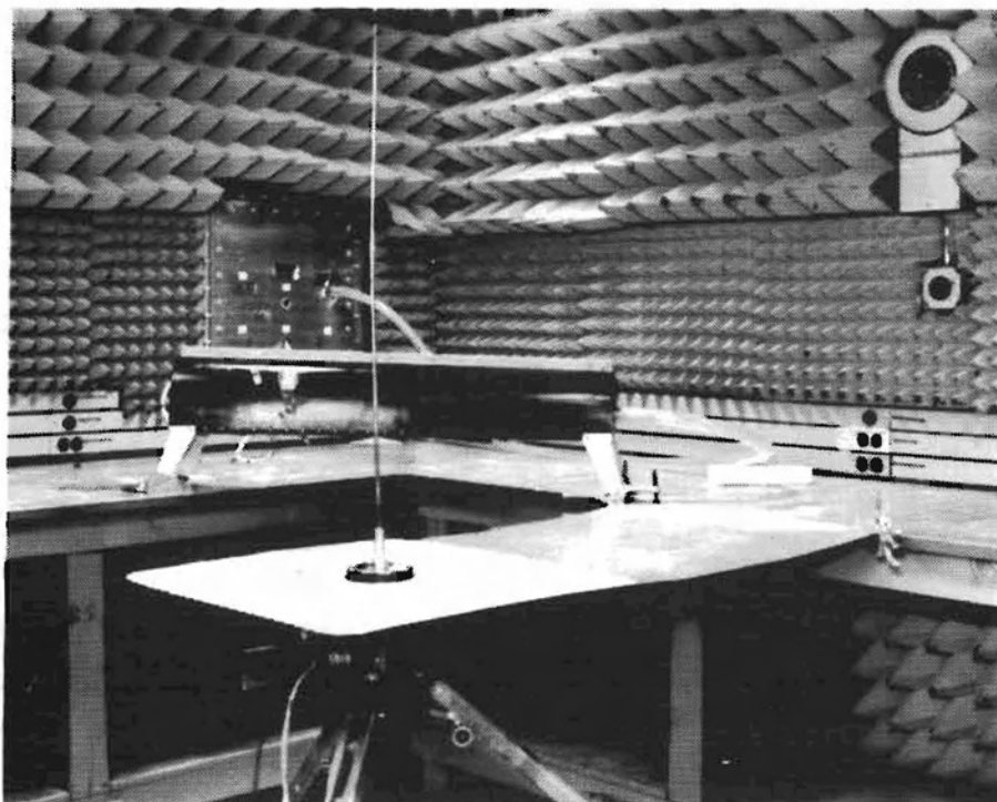
Figure 3-9 First Test Setup for Composite Wing
