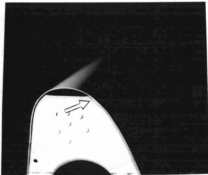
Figure 2-5 Hairline Crack on End Rib (Crack is at Upper Right Corner of Rib) (0.025-Inch Skin)
