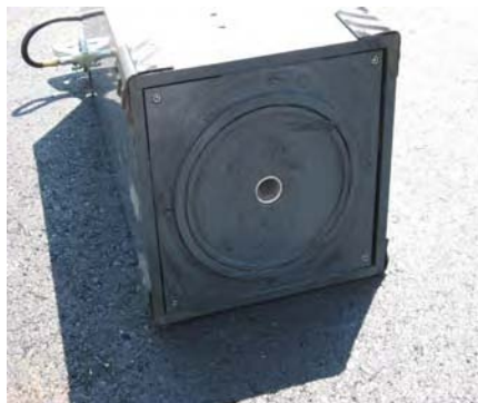
Figure 2: Air Permeameter Grease Ring
