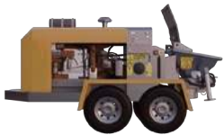
CONCRETE PUMP WITH HOPPER
