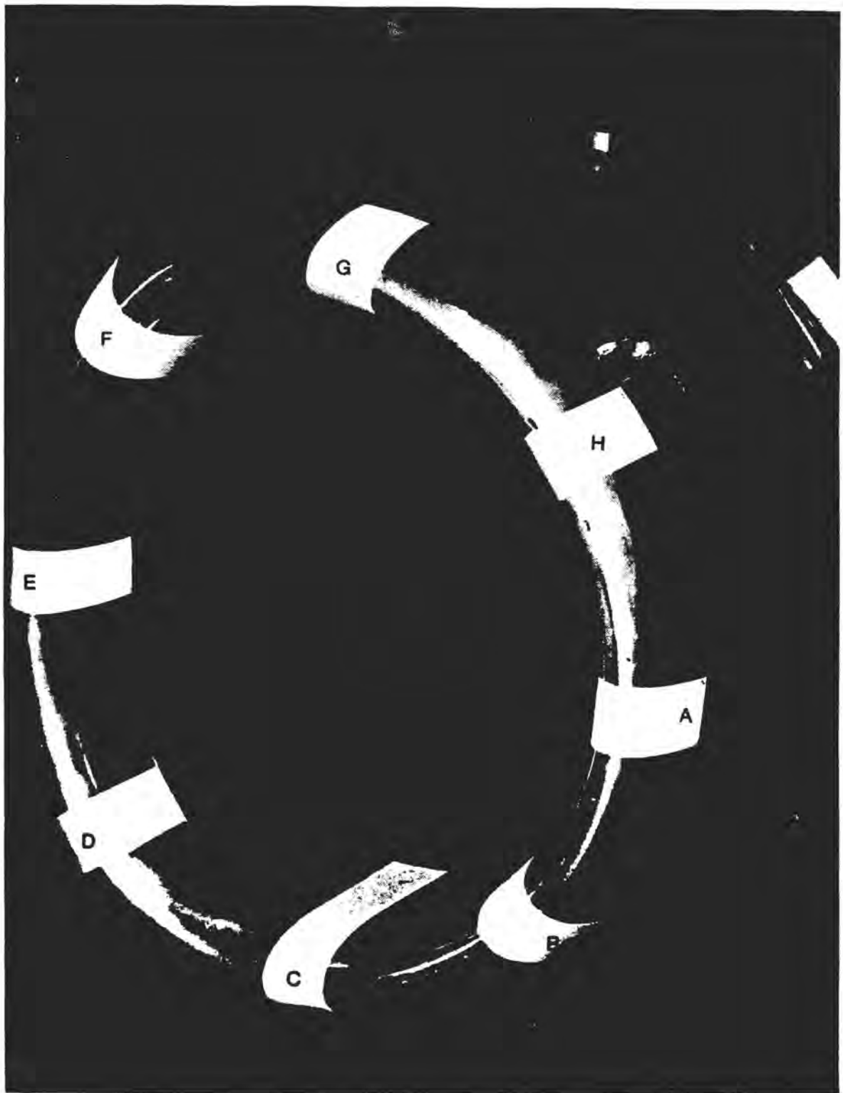
FIGURE 2-32. BLOTTER STRIP LOCATIONS ON BOEING 737-300 INLET FOR \alpha = 0^\circ AND \alpha = 15^\circ TESTS (REFERENCE 2-15)
