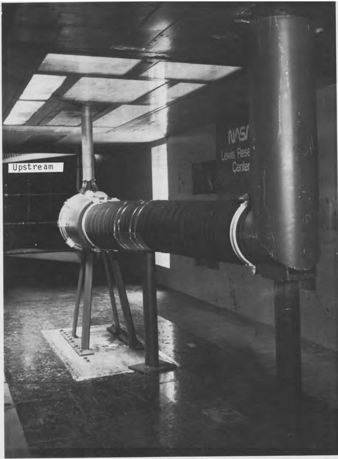
FIGURE B.8 ENGINE INLET CONNECTED TO THE NASA SUCTION SYSTEM.
