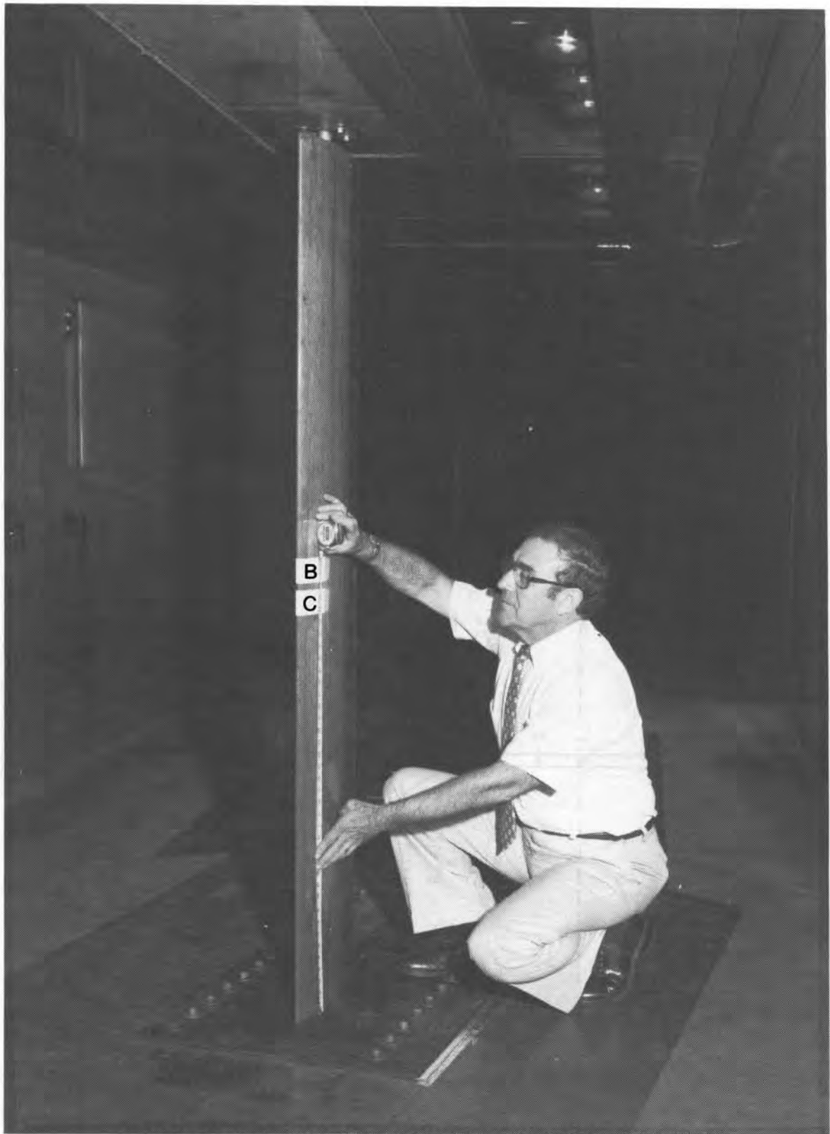
NACA 65 2 015 AIRFOIL WITH BLOTTER STRIPS INSTALLED
