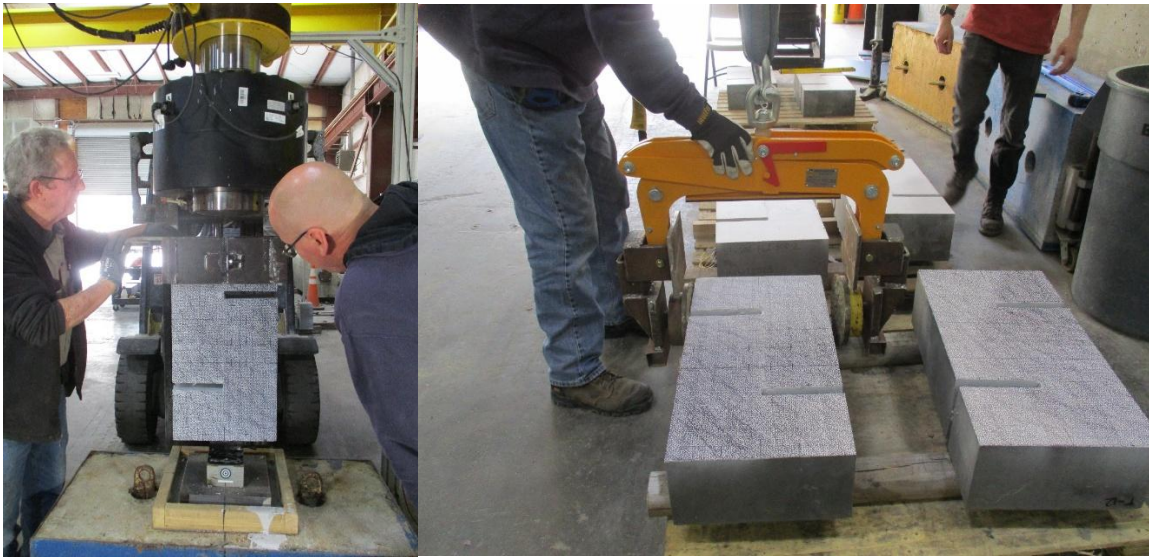
Photo 2.12. Handling of large UHPC pushoff test specimen by forklift and crane.
