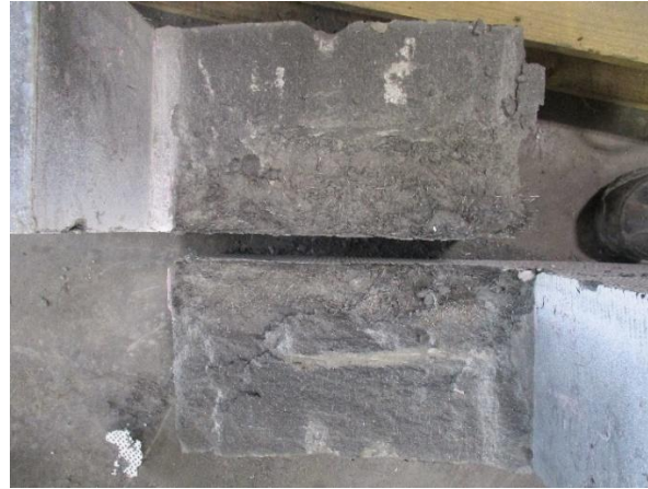
Photo 4.2. Segregated fibers in Set 0 pushoff specimens.
