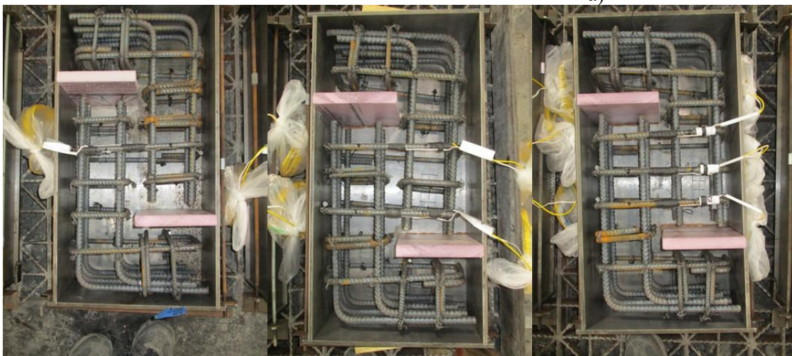
Photo 2.2. Placement of rebar strain gage and fiber optic strain gages on a) matchcast pushoff specimens and b) monolithically cast specimens.
