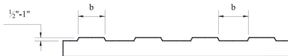
Figure 1.18. Fluted interface proposed by Tadros et al. [5] for UHPC-to-UHPC interfaces.
