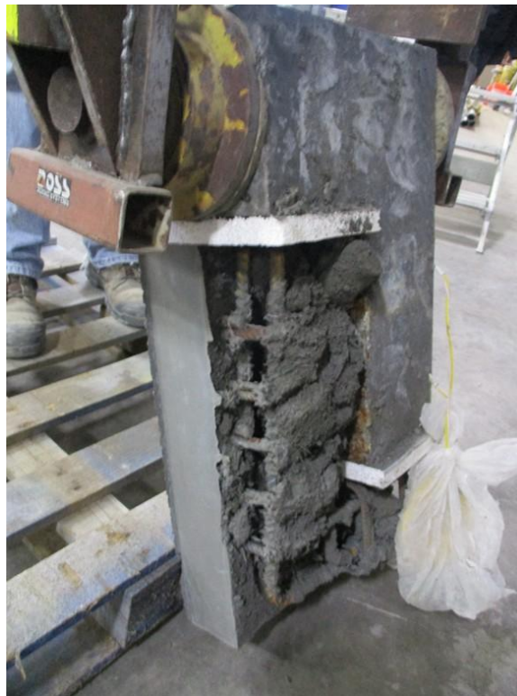
Photo 7.2. Poor workability material due to water underdosage
