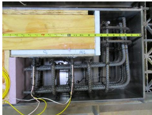
Photo 2.1. Reinforcement crossing shear plane on shear pushoff test (left: \rho_v=0 and right: \rho_v=9.2e-3 ).
