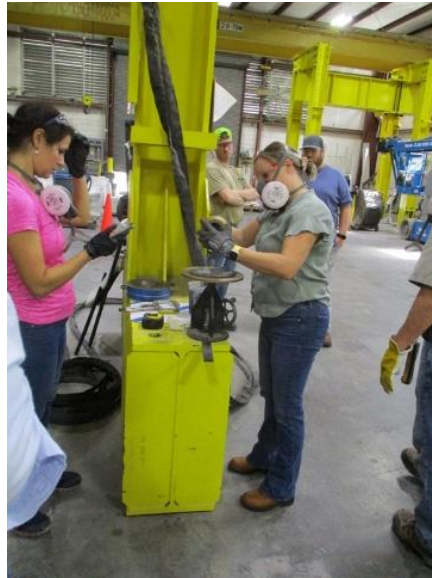
Photo 2.8. UHPC flow table test.
