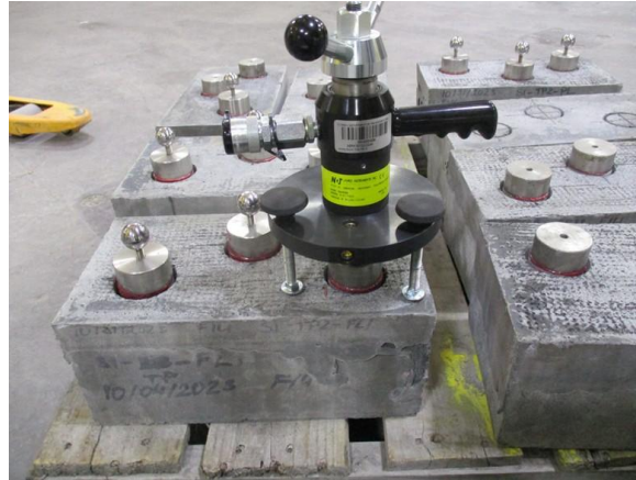
Photo 4.1. Pulloff test device.
