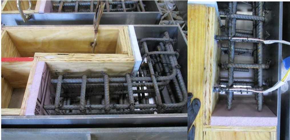
Photo 2.1. Reinforcement crossing shear plane on shear pushoff test (left: \rho_v=0 and right: \rho_v=9.2e-3 ).
