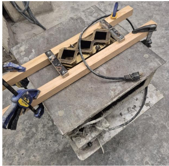
Figure 4-28: Restraining Device Used to Prevent Mold Movement During Vibrating Table Consolidation
