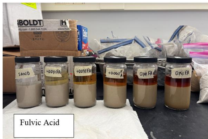
Figure 4-35: AASHTO T 21 Results with Controlled Additions of Fulvic Acid
