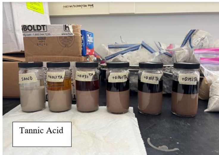
Figure 4-34: AASHTO T 21 Results with Controlled Additions of Tannic Acid
