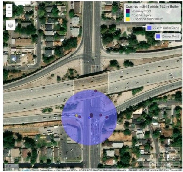
Figure 36: Influence area at diamond interchange ramp terminals (I-80 700 E)
