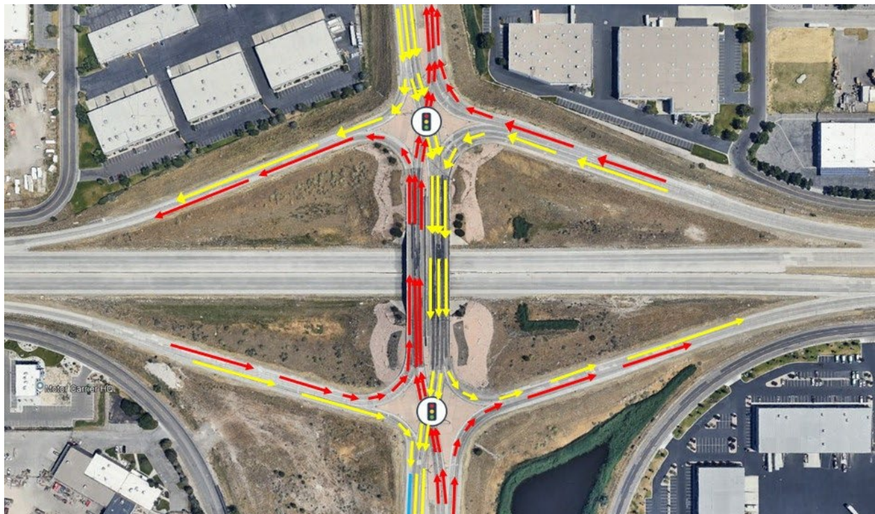
Figure 1: Traffic movements at a typical DDI (SR-201 and Bangerter Highway, Utah)
