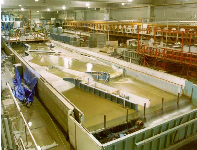
Figure 4.6. Photograph of hydraulics laboratory with river model during testing (center of photograph).
