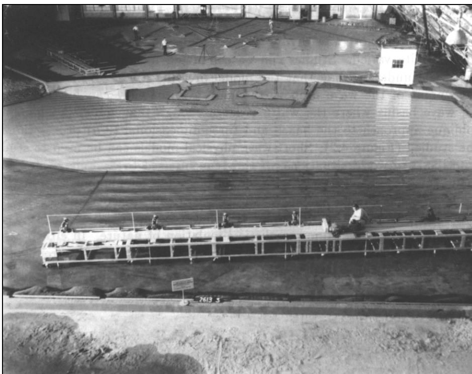
Figure 4.8. Typical laboratory wave basin (Hughes 1993).
