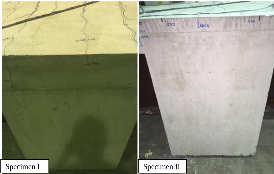
Figure 39. Diaphragm cracks on long side for each specimen
