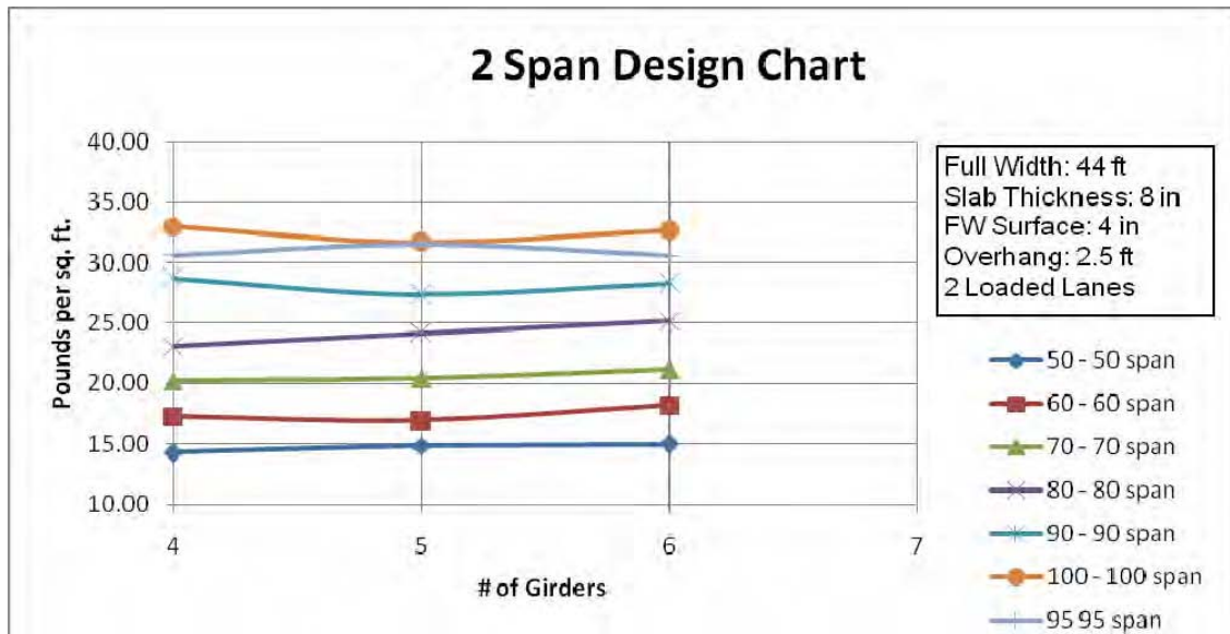
Figure 4-2: Linear Interpolation Between a 90 ft and 100 ft Two Span Bridge
