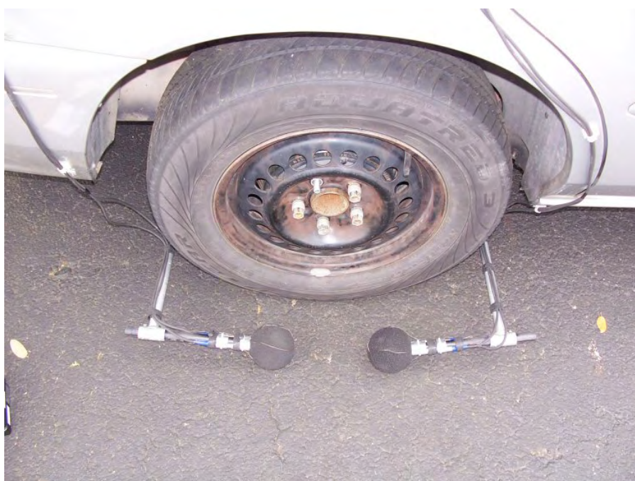
Figure A.2. OBSI Measurement Bracket Configuration.
