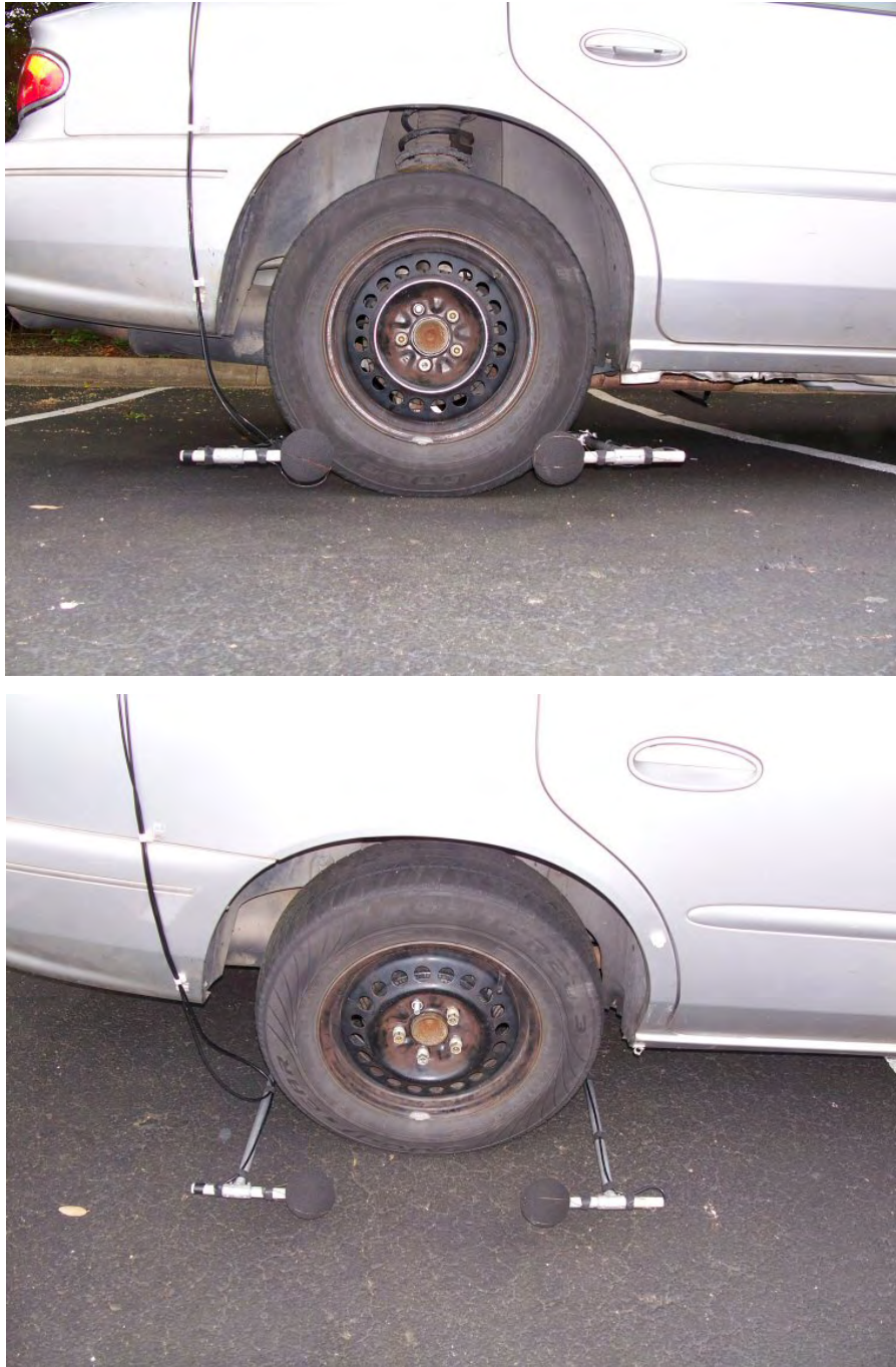
Figure A.1. CPX Measurement Bracket Configuration.
