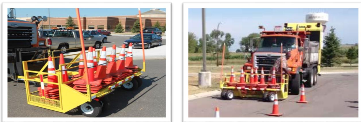
Figure 21. MnDOT TTCD cart (47).
