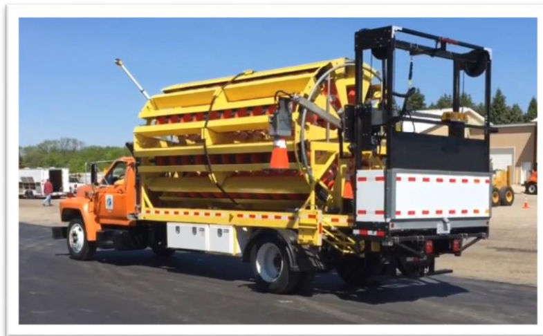
Figure 5. MnDOT AutoCone 500 truck (16).
