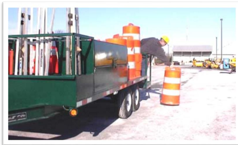
Figure 8. Centreville Roadway Workzone Safety Trailer (25).
