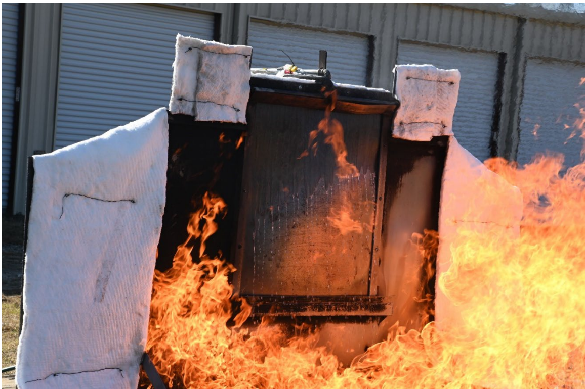
Pool fire test – activating cooling water
