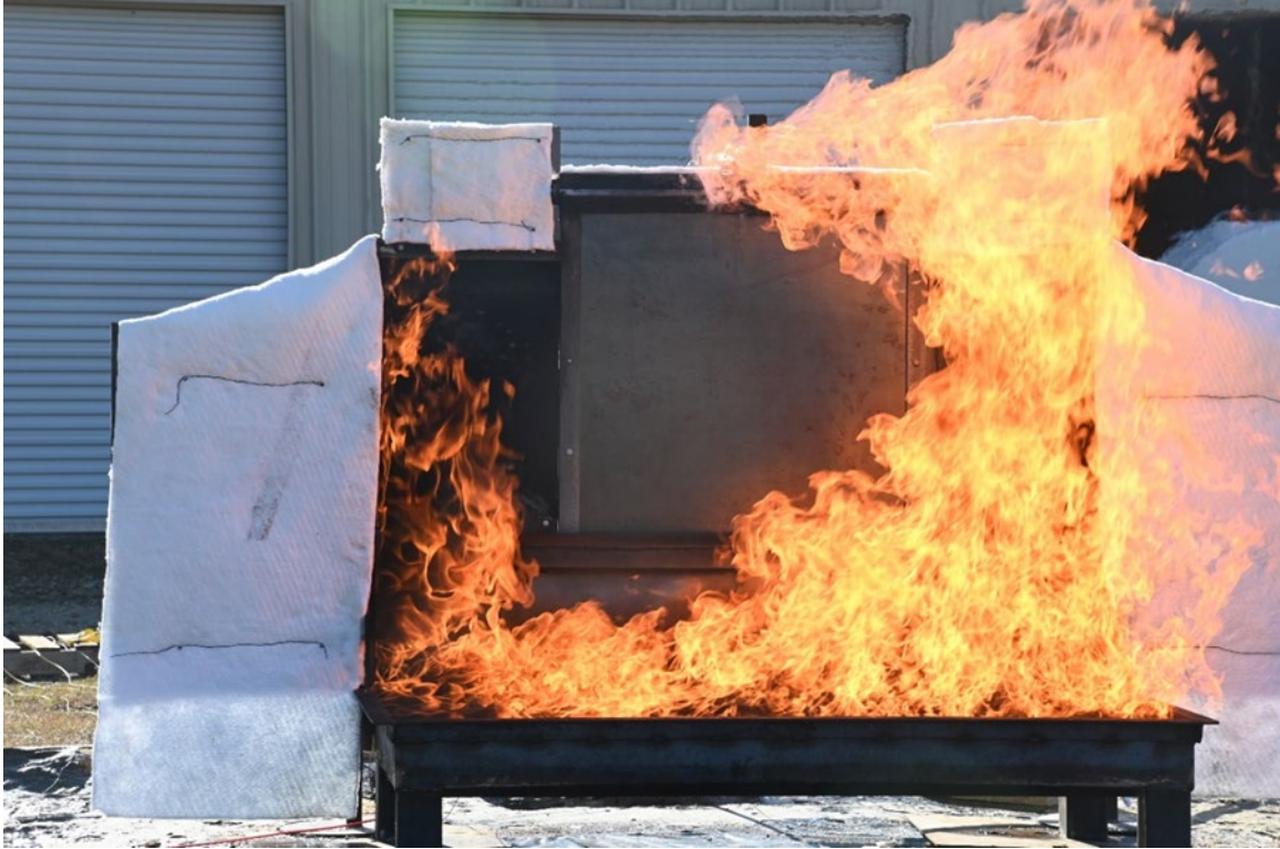
Pool fire test before cooling water
