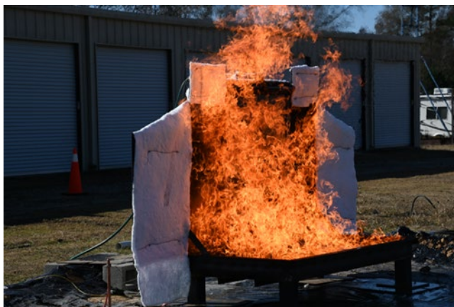
Figure 29. Ethanol pool fire experiment before activating cooling water
