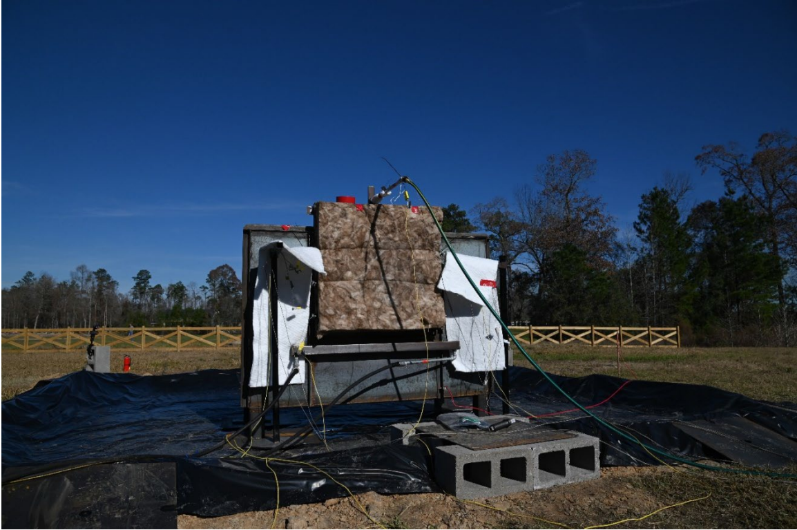
Pool fire test apparatus – back (protected side)
