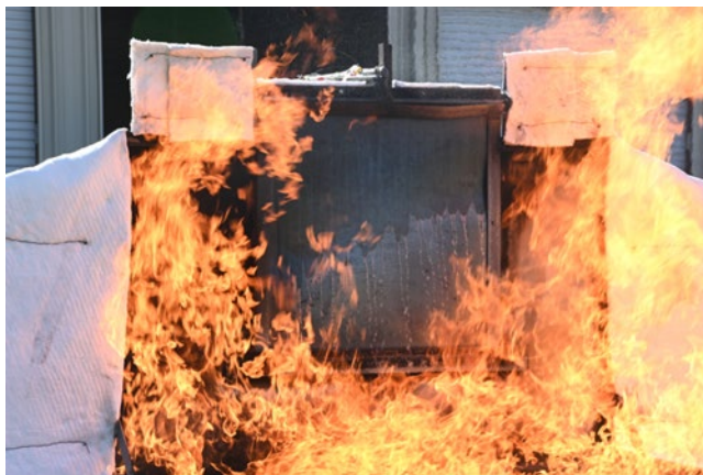
Figure 30. Ethanol pool fire experiment after activating cooling water
