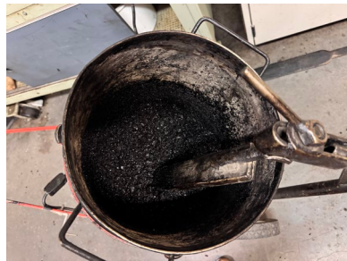
(a) mixing the aggregates and asphalt binder
