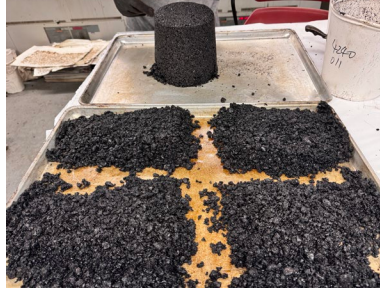
Figure 3-1 breaking down and quartering the reheated plant-produced mixtures
