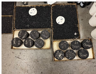
Figure 3-3 Compacted and loose LTA conditioning
