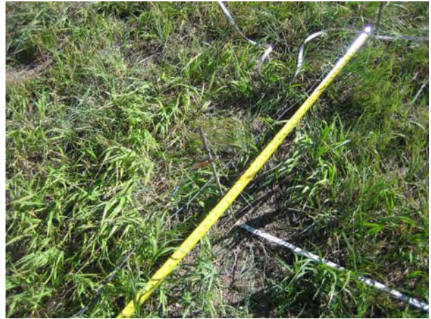
Figure 9. Field measurement of soil resistivity
