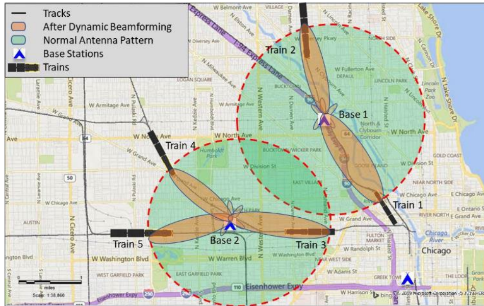
Figure 17. Implementation of smart antenna system at base station platform
