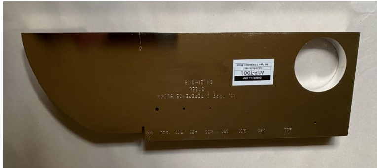
Figure 6. IIW Type 2 calibration block
