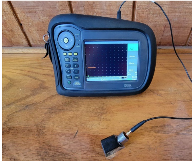
Figure 5. Typical ultrasonic wedge, transducer, cable, and detector
