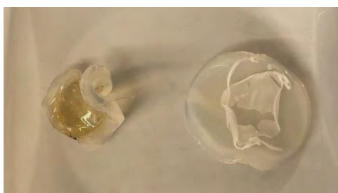
Figure 3.7: Imperfections in polyurethane coating observed after 6 hours of immersion. Oil-based and water-based coating shown on left and right, respectively.
