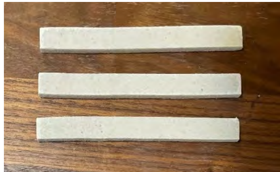
Figure 2.13: Samples created for BBR testing by mixing agar-based binders with Ottawa sand at a ratio of 2:1. Representative specimen for A5-L agar-based binders measuring 0.5 in wide and 6 in long.
