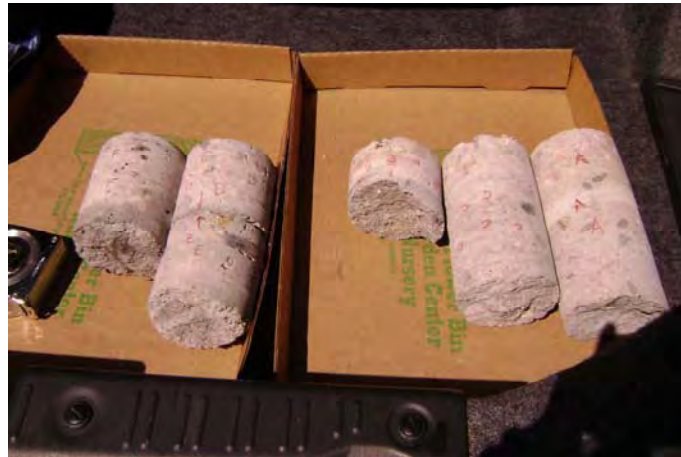
Figure 3-4 Coring samples on Bridge G-22-BH
